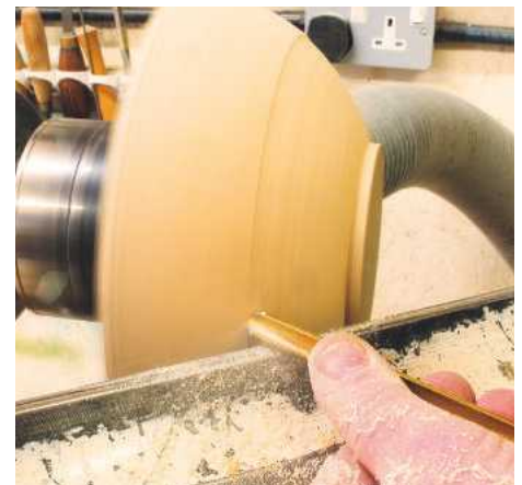
▲ Pic.9 Once the shape is roughed out with the 13mm gouge Les goes to the 10mm bowl gouge for his finishing cuts. This is a push cut with the bevel rubbing and will give a great finish
